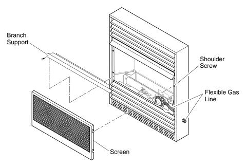
Figure 24 - Removing Log Base Assembly From Fireplace
